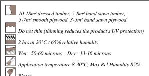
use. Its woodstain like qualities ensure timber grain remains highly visible. Cetol BLX-Pro is microporous allowing the timber to breathe.
